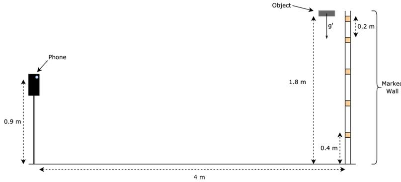
Figure 1: A diagram showing the experimental setup, including the exact distances and positions
